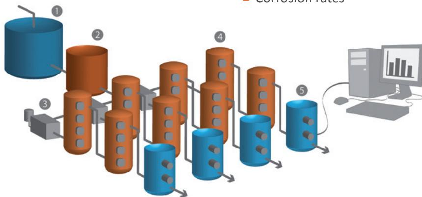
① Nutrients    ② Chemostat (tank of active microorganisms)
